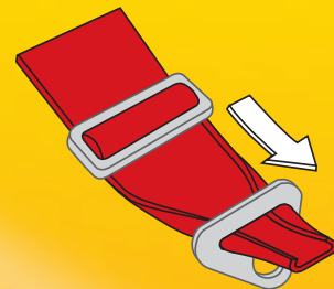
STEP 2: Pull strap to 8"-10" beyond buckle, fold edges and insert into mounting bracket.
